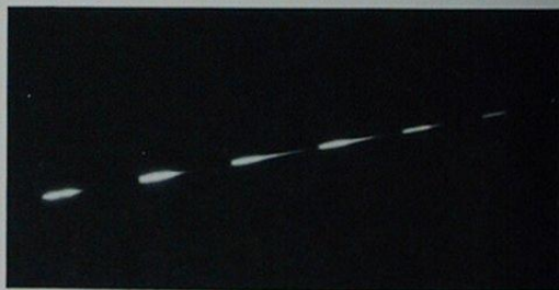
A bright meteor trail recorded at one of the twelve field stations of the Meteor Observation and Recovery Project which is operated by NRC in the prairie provinces. The trail image is chopped 3 times per second by a rotating shutter to provide velocity and deceleration data. This meteor trail is about 25 km long at an altitude of about 90 km. Such meteors very often generate UFO reports.
