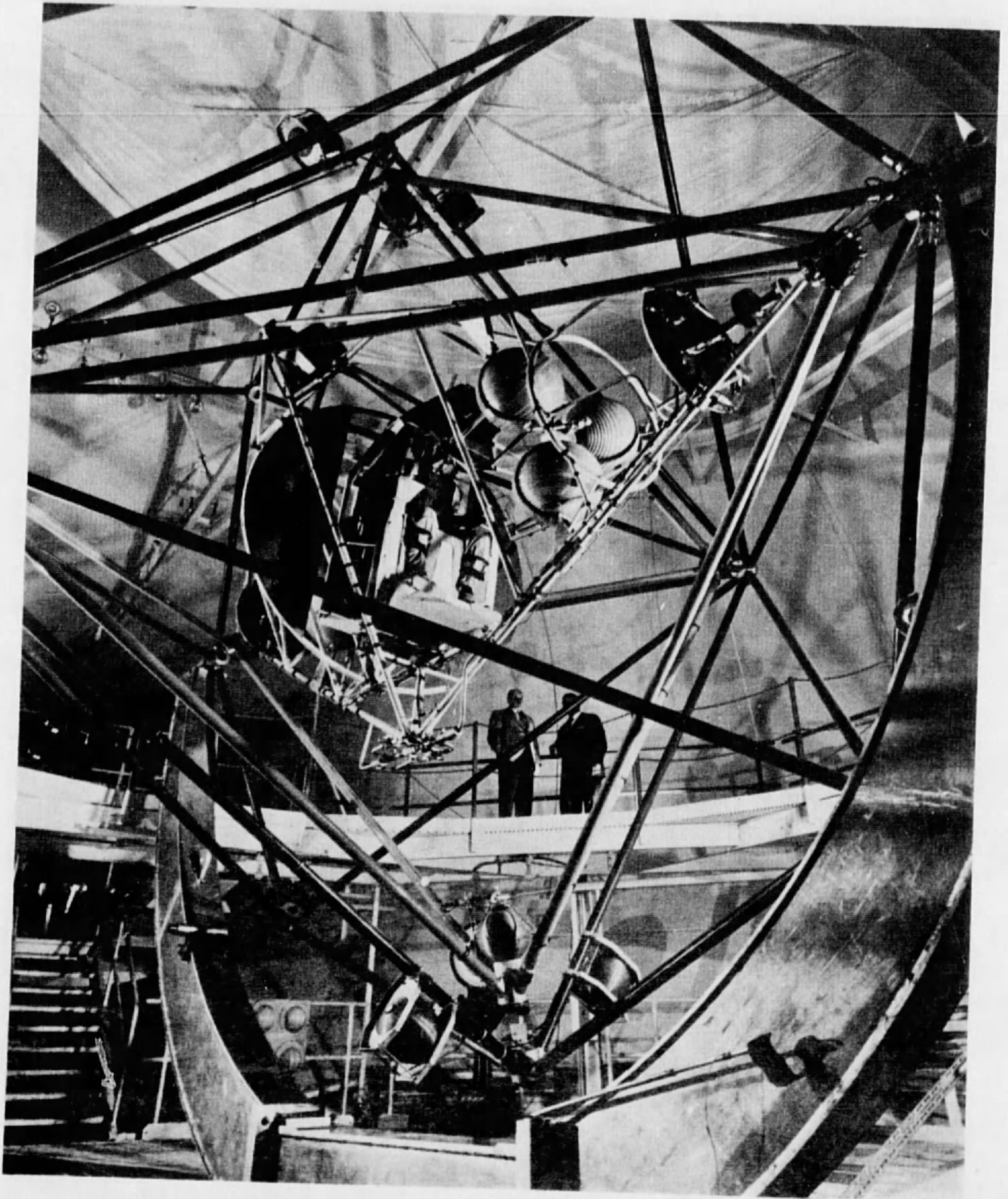
FIGURE 30.—Multiaxis motion simulation at Lewis research center.
