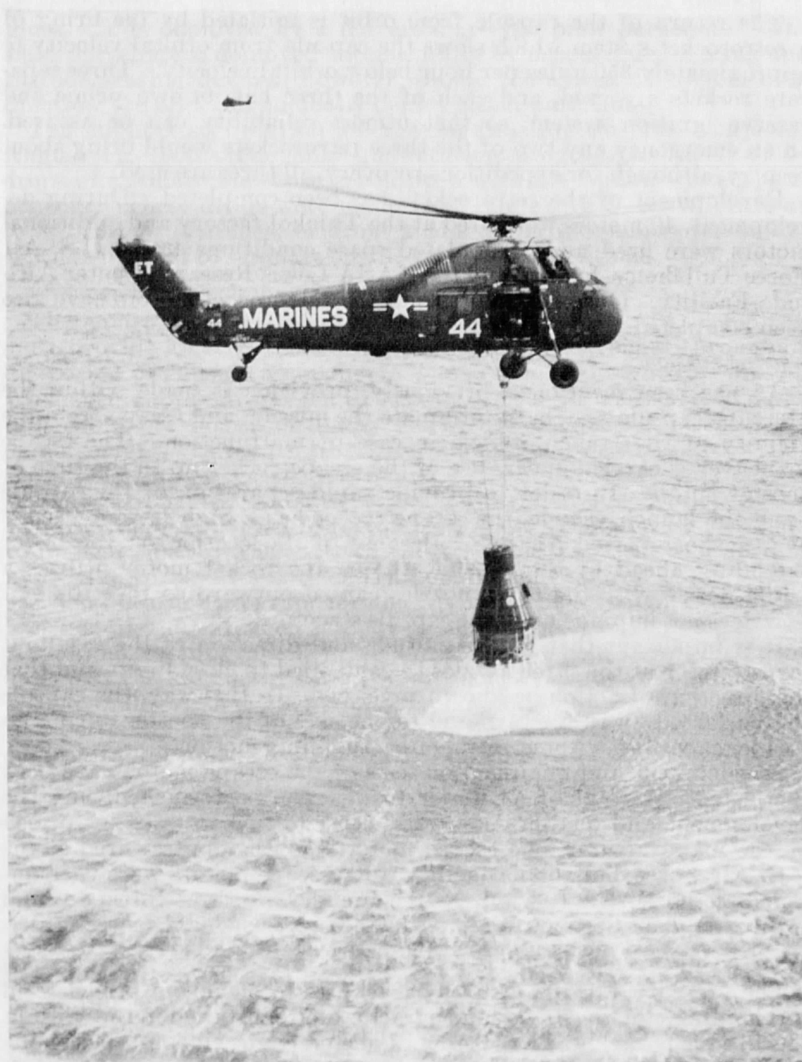
FIGURE 5.—MR-3 capsule with extended impact bag.
