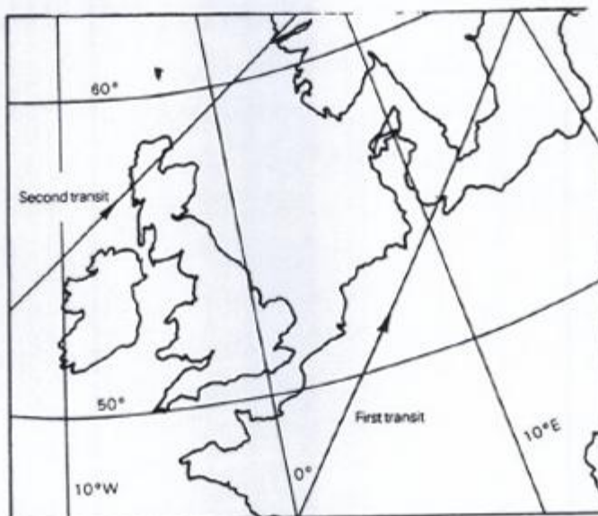
Figure 7: 90 Minute Orbit Tracks at 65° Inclination (U)
